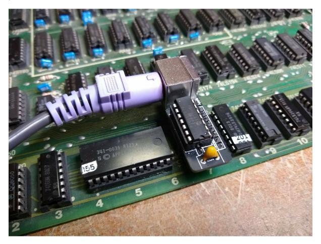
Check if the adapter pins are fitted well in the socket and that no pins are bent.
