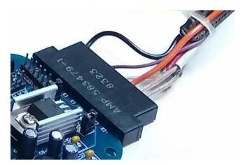
**10-wire connector** (a jumper over pins 3 and 9 is required):
